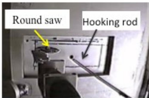
(1) Photograph of opening the aluminum plates of TMRA and Cd liner window of cold moderator shown in Fig. 2(2) .
