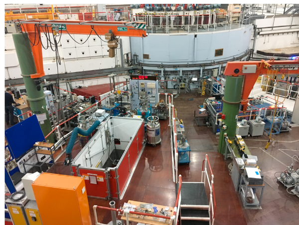
Fig. 5. Photograph of one side of the ISIS pulsed spallation source. The light-blue circular enclosure contains the spallation target, with the proton beam coming from left to right. The motors on the top of the target enclosure control the shutters for the various beams. Most instruments are hidden below the floor, but the red enclosure gives access to the top of the POLARIS diffractometer. Photograph by MTD. (For interpretation of the references to colour in this figure legend, the reader is referred to the Web version of this article.)
