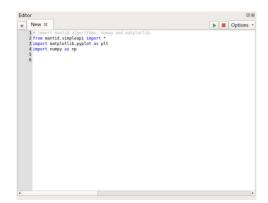
To run a script, either hit the green arrow or select options, hit "Ctrl+Shift+Enter" and hit "Run". There are more options available to the user, such us "Abort" to stop the execution." Run All" will run the whole script. To run part of the script, highlight the desired part and hit "Run".
